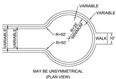
NOTE: FOR FIRE TRUCK CLEARANCE, NO OBSTRUCTION TALLER THAN 6" SHALL BE PERMITTED WITHIN 3FT. OF THE CURB. ON-STREET PARKING SHALL BE PROHIBITED.
