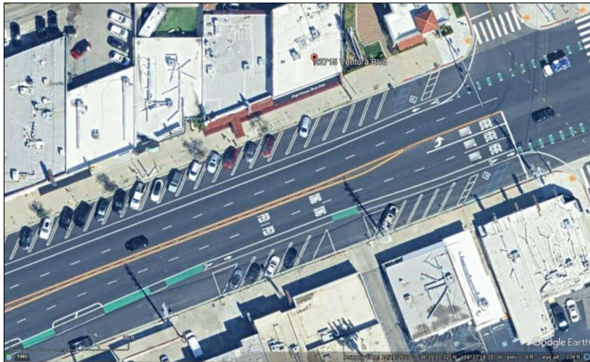
22000 Block of Ventura Boulevard Diagonal parking with back-in parking (21' parking + 6' bike lane = 27' to travel lane) Total street width: 100'
